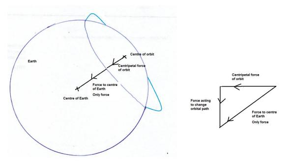
To maintain a circular orbit, the sum of the physical forces must produce the centripetal force. Gravitational forces push a satellite towards the centre of mass of the Earth, thus this must also be the centre of the orbit.
