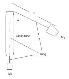
A student holds the glass tube and swings the rubber stopper  $(M_1)$  in a circle maintaining a constant radius. The force (tension in the string) is provided by the mass  $(M_2)$ . Another student measures the time taken for 25 revolutions.
