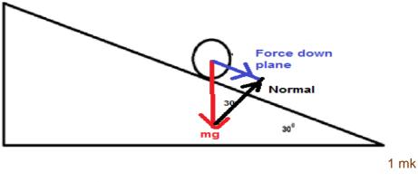
Normal =  $\cos 30^{\circ} x \text{ mg} = 0.8660 \text{ x} 2 \text{ x} 9.8 = 17.0 \text{ N}$ 1 mk 1 mk
